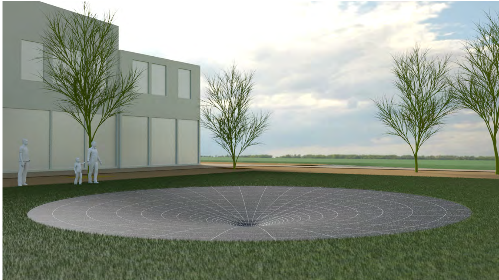
Black terrazzo surface with embedded aluminum profiles in grass landscape
